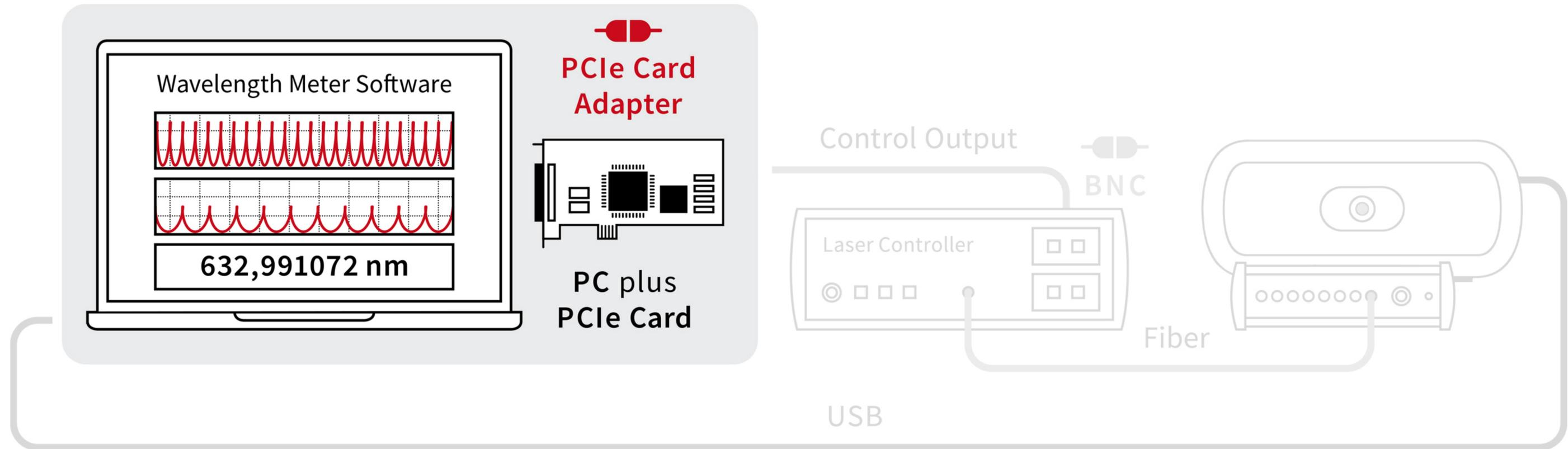
Insert the PCIe card to a suitable PCIe slot on your computer and **install the wavelength meter software** (which installs all drivers automatically).
