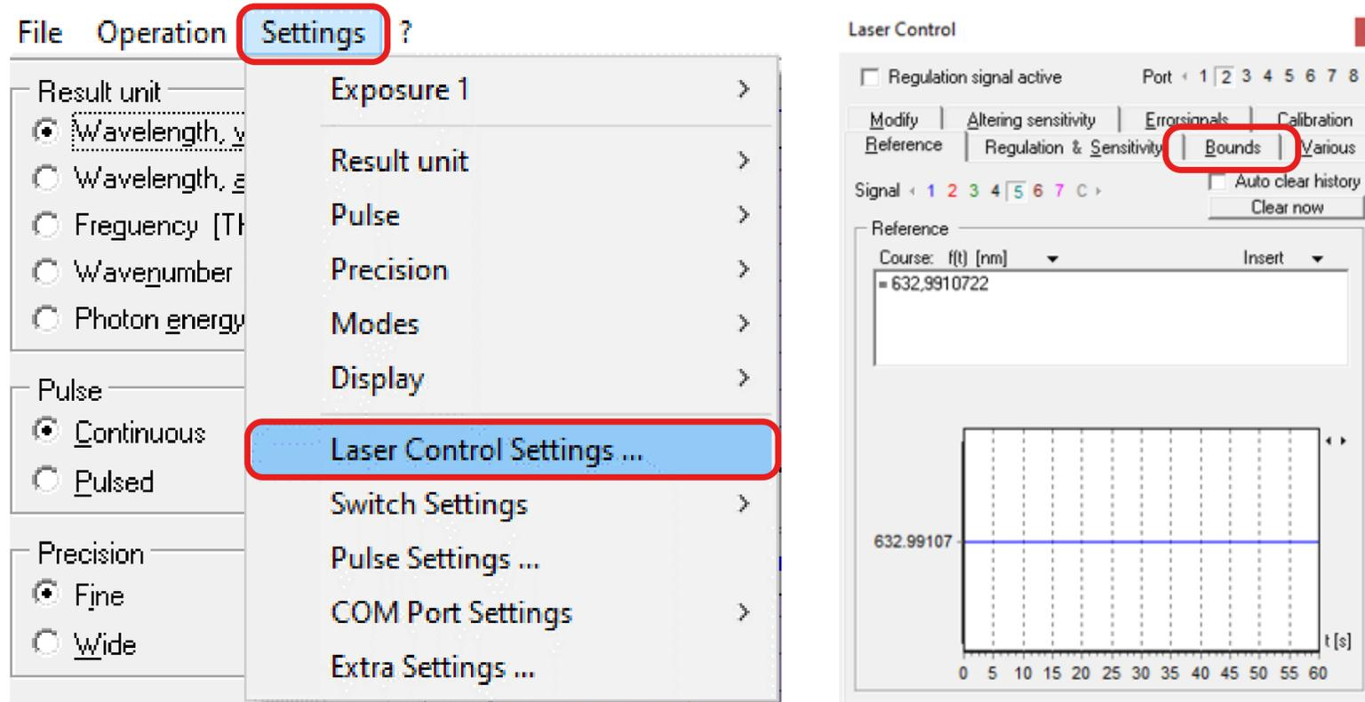
Start the software and set the voltage bounds in the Laser Control Menu such that you can exclude a damage to your laser and make sure the output range is suitable (e.g. as defined by a mode-hop-free scanning range).
