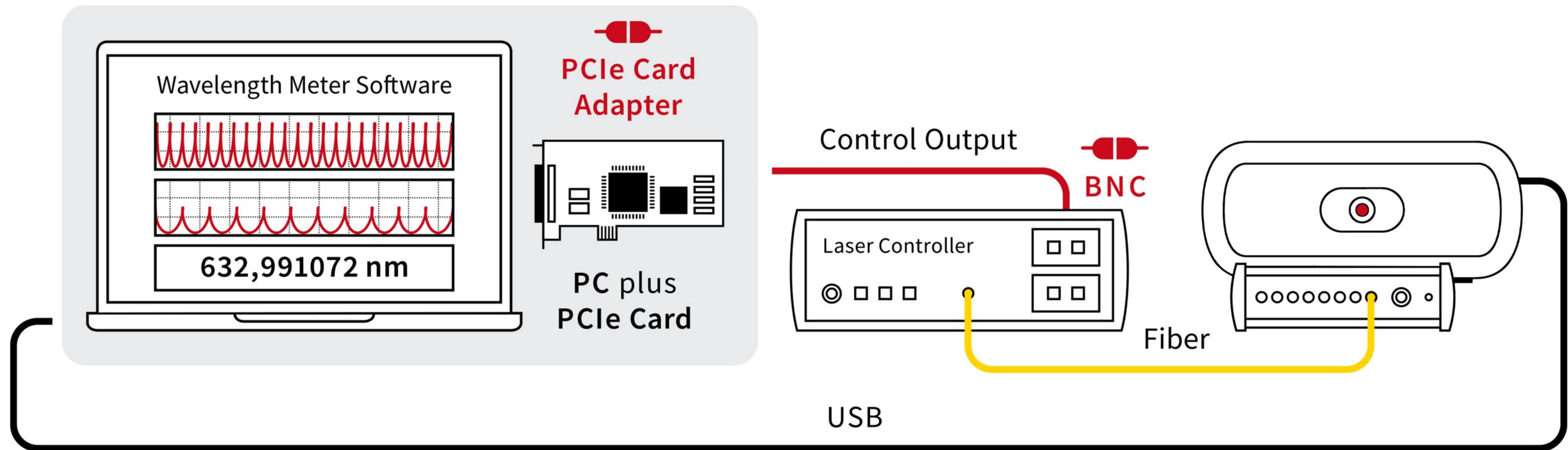
Connect the voltage output of the PCIe card to the input at the laser using the adapter cable (minimum impedance at the laser input 10 kOhm).
