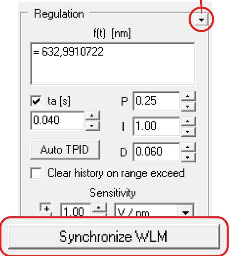
The tool can be used as a **pure simulation** tool or **synchronized to the wavelength meter software** running in parallel.
