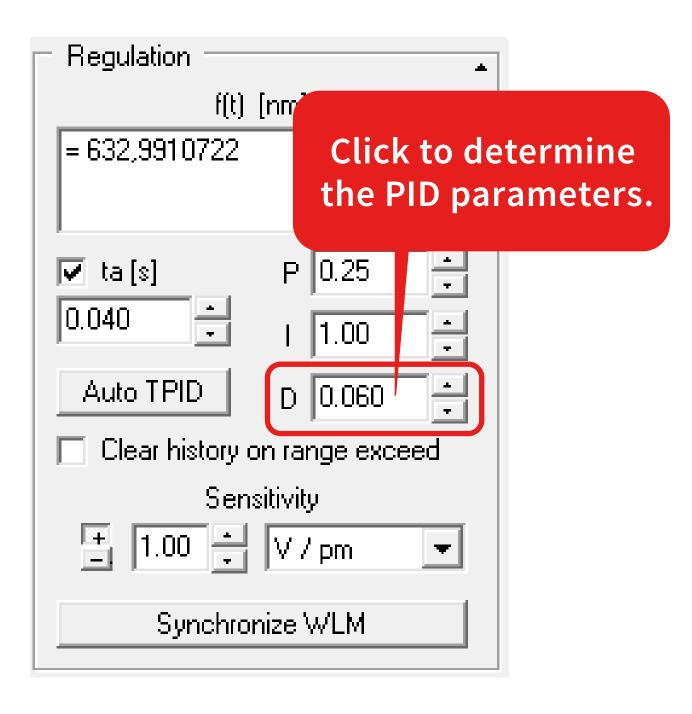
Press "Auto TPID" to determine the PID parameters. Finally, you can close the PIDSim2. Now the system should be ready for a test.
