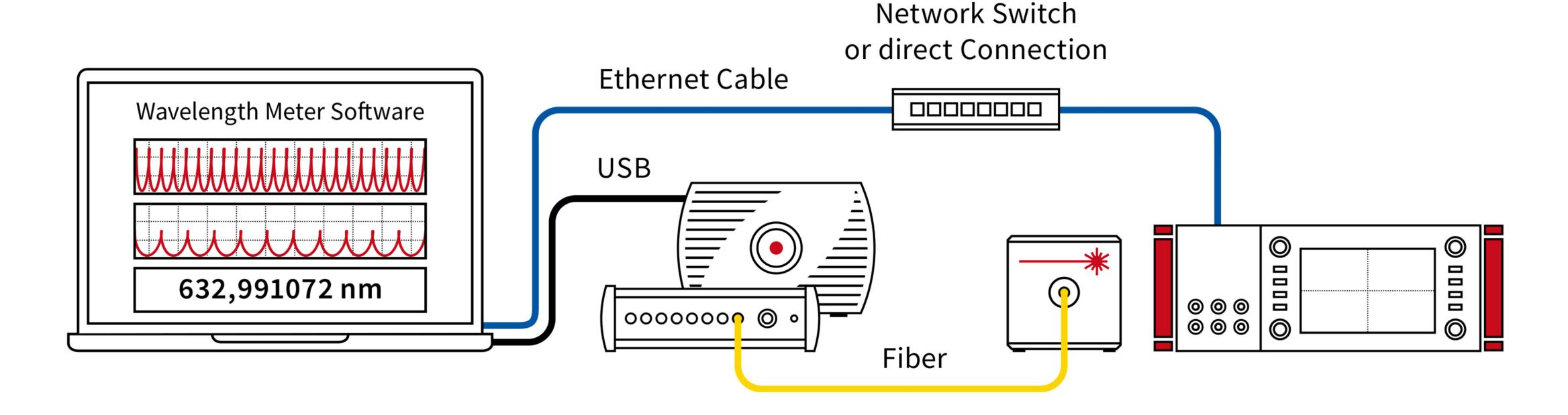
Connect the DLC pro Controller and the computer running the wavemeter software to the same network (UDP has to be allowed for automatic recognition).
