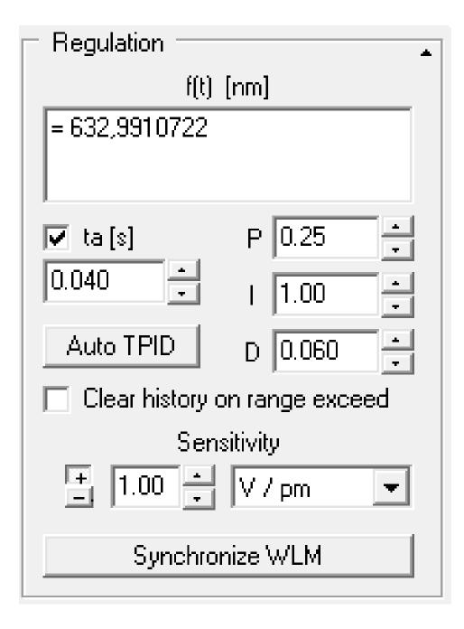
In this example the laser should be stabilized at 632.9910722 nm.
