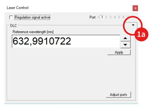
Start the software and set the voltage bounds in the Laser Control Menu such that you can exclude a damage to your laser and make sure the output range is suitable (e.g. as defined by a mode-hope-free scanning range).
