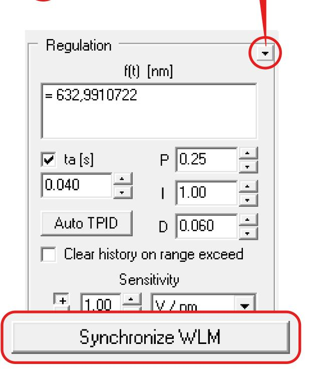
The tool can be used as a pure simulation tool or synchronized to the wavelength meter software running in parallel.
