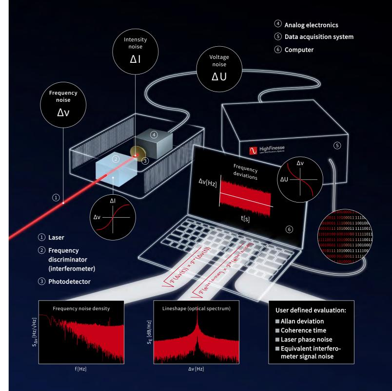
The laser light ① is coupled to the input fiber and lead through an interferometer ② acting as a frequency discriminator. The transmitted intensity, which is directly proportional to the variations of the input frequency, is converted by a photodetector ③ and our analog electronics ④ into a voltage signal.
