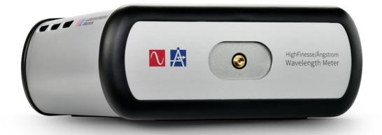
The optical unit consists of Fizeau-based interferometers which are read out by photodiode arrays. We achieve remarkable high accuracy and stability by using exclusive, non-moving optics.
